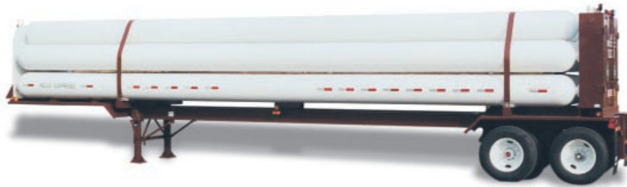
Figure 74. Tube trailer for gaseous hydrogen truck delivery. 60
