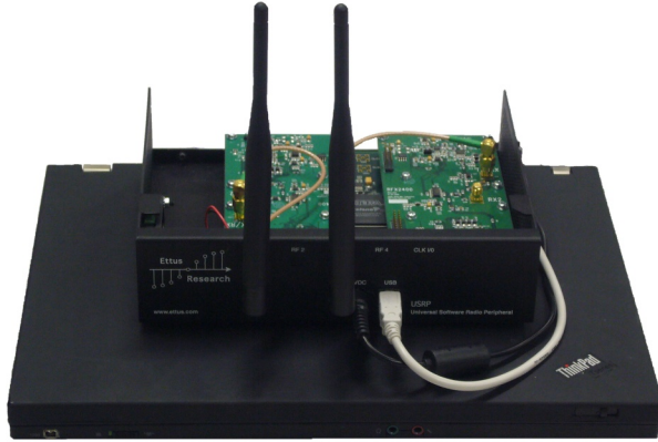
Figure 8.1: Hardware setup of our UFH prototype, consisting of a Universal Software Radio Peripheral (USRP) and a Lenovo T61 ThinkPad.
